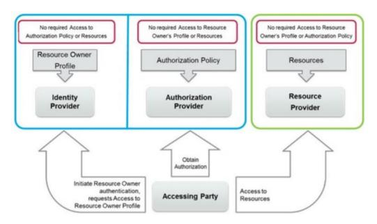
Figure 1: The Separation of Duties Principle
