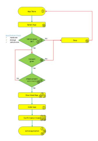
Figure 28: Installing an Application in the Vehicle
