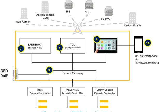
Figure 5: Secure OTP On-board Architecture
