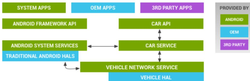
**Figure 1.** Vehicle HAL and Android automotive architecture
