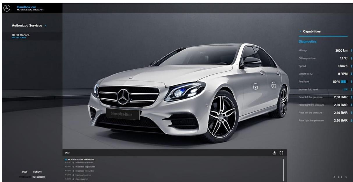
Figure 6: The sandbox car and the Diagnostics capabilities of Mercedes ExVe
