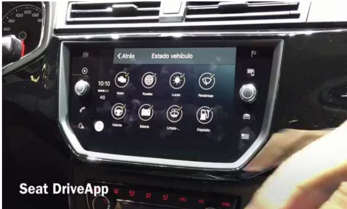
Figure 10: Seat App from 2016, using the OEM version of Apple CarPlay (taken from 2018 study)
