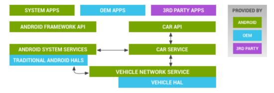
The vehicle HAL is the interface definition between the car and the vehicle network service:
